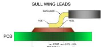
Fig 3 SMT Lead on surface
