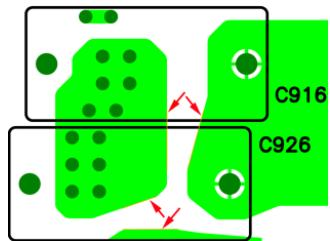
Fig 7 Arc-stopping Gaps
