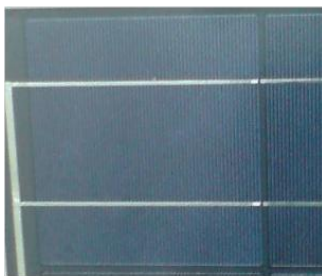
Fig. 10a: Can you see the microcrack in this new cell?
