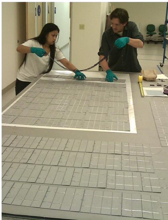
Fig. 13: An idealPV solar panel is assembled from low cost, low reverse breakdown solar cells.
