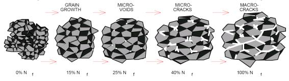
Figure 1: Depiction of the Effects of the Accumulating Fatigue Damage in Solder Joint Structure [1].
